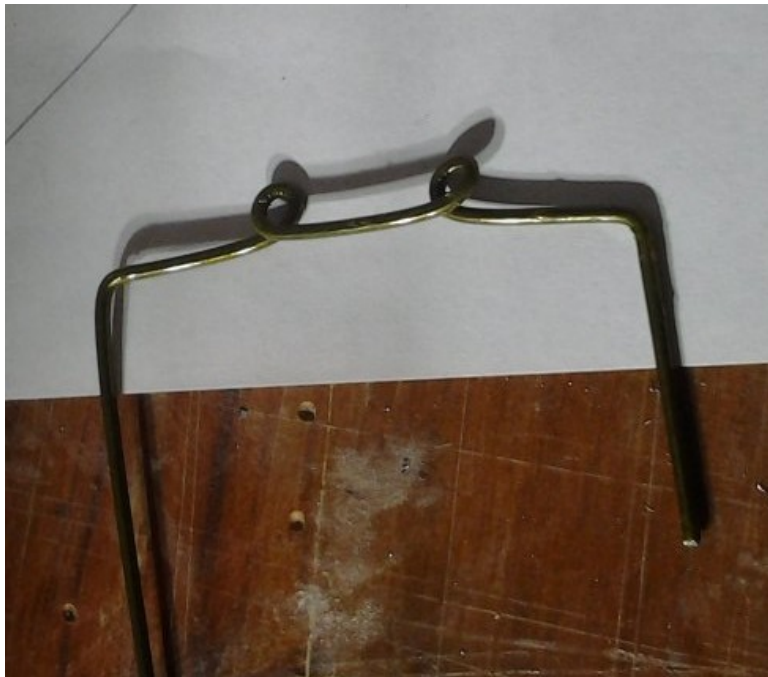
Figure 25: Bend to make the prongs
