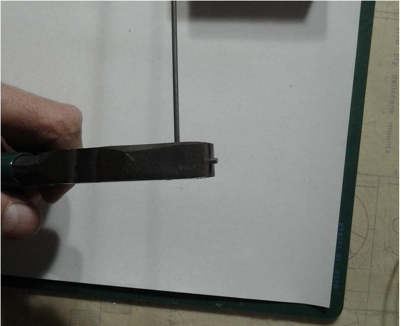
Figure 20: Z bend: second, bend the wire towards you through 90 degrees.
