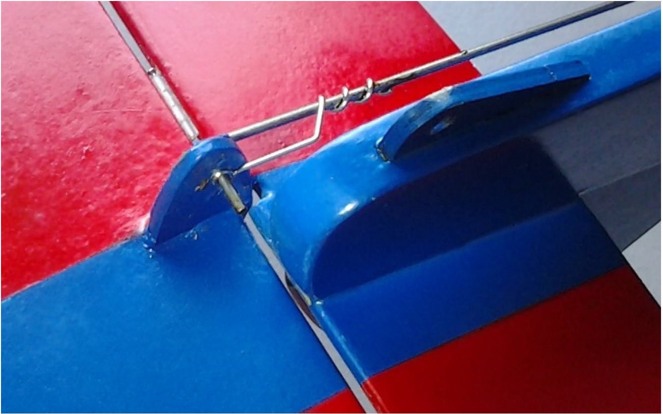
Figure 23: A pushrod held on with a retainer
